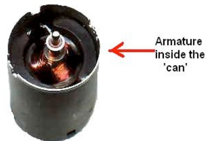
Photo #3 is the armature inside the can.
